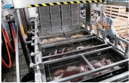
一所著名的本地快餐連鎖店在其中央廚房安裝了自動的液態浸漬冷凍系統。 One of Hong Kong's most well-known fast food chains has installed an automated liquid immersion freezing system in its master kitchen.
